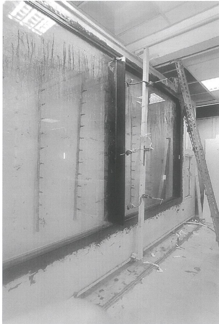
Figure (4): Photo of SLIM-X LITE sliding window system during structural performance test
